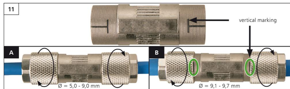
Demontage / Disassembly / Demontage
